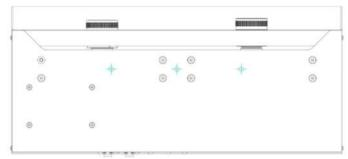
▲The bottom plate of the 4000-D series – 1/4" UNC in the middle and M6 screw holes
