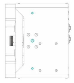
▲The bottom plate of the 2000 Series - 1/4" UNC in the middle and M6 screw holes
