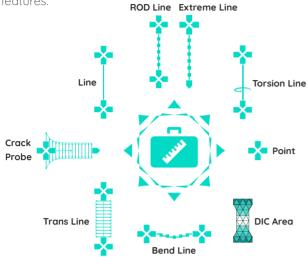
The VE typically includes an AXIAL software module. The measurements with VE are primarily performed in real-time using line-based measuring probes with online data transfer to the testing machine.
