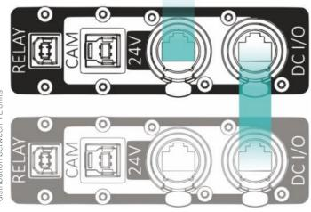
The DC I/O port can be used as an alternative power  $\ensuremath{\text{INPUT}}$  In such a case, the power is distributed directly to the LED light, bypassing the USB relay.
