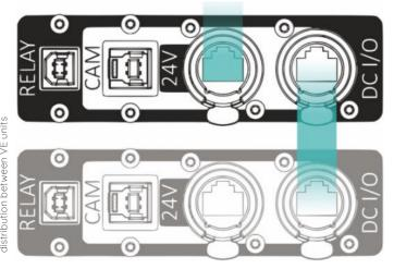
The DC I/O port can be used as an alternative power **INPUT** In such a case, the power is distributed directly to the LED light, bypassing the USB relay.
