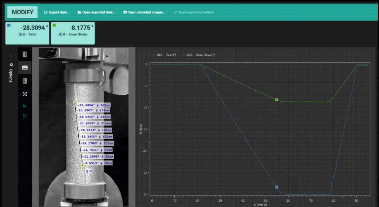
The evaluation of Twist and Shear Strain in degrees by using the Torsion Line tool.
